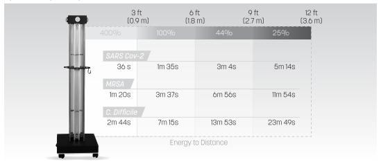
The table above shows the run times needed for the targeted pathogen reduction at the distance from the T80 tower. The results were obtained by measuring the power of UV-C light at specific distances. The power in [mW / cm $^2$ ] multiplied by the time unit [s] makes it possible to calculate the radiation dose in [mJ / cm $^2$ ].
